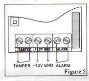
TAMPER TEMPER OUTPUT PORT +12V DC ANODE GND DC CATHODE ALARM ALARM OUTPUT PORT
