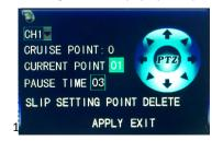
Operate the PTZ with mouse through the keypad on the interface. Set the cruise point in the cruise setup, as shown on the right picture above.
