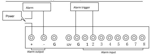
Note: The above picture is the type of normally on alarm, and normally off is the opposite way.
