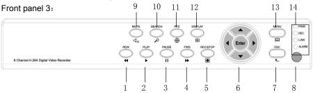
1.Rewind 2.Play 3.Pause 4.Forward 5.Manual start/stop recording 6.up,down,left,right and Confirm 7.ESC:Exit/Return 8.Remote control infrared receiver 9.Mute 10.Video search 11.PTZ control 12.DISPLAY:Display mode 13.MENU:Main menu 14.Status indicator
