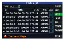
The backup of recording files can be achieved through USB storage device. Before backup, the user must insert storage peripheral devices to USB2.0 slot first. Move the cursor up and down in the interface of detailed file list and select "Backup". The file is undergoing backup and the
