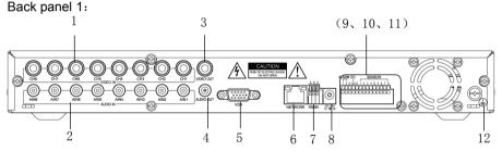
1.Video in 2.Audio in 3.Video out 4.Audio out 5.VGA video output port 6.Network port 7.RS485 8.Power supply 9.Alarm output 10.Auxiliary DC12V output 11.Alarm input 12.Grounding terminal
