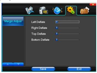
By the function, you can adjust the distance between the display device and the picture edge.
