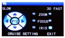
PTZ speed (fast or slow) can be controlled in this interface, zoom, focus and aperture is also controllable.
