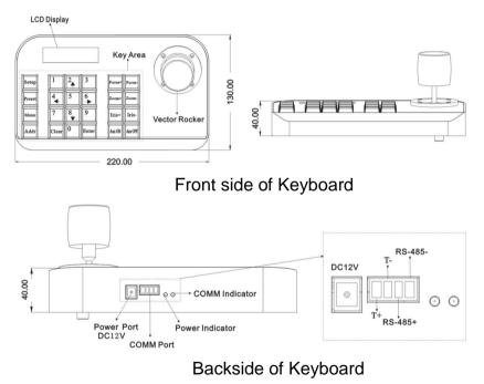
Power Supply Interface: Connect to external stable voltage DC12V input through this interface.
