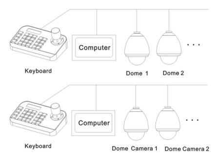
Notice: Before using the keyboard to control dome camera, please make sure the address, protocol, baud rate of the
