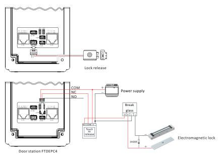
🕲 This device comes with a varistor. A varistor (or diode) must be connected across the lock terminal as the varistor controls the overload produced by the strike coil or maglock. If not used then this may cause inerasable damage. If a maglock is to be used then an extra PSU, break glass, push button to exit may be required. Please arrange according to your need.
