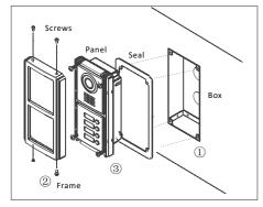
a. Cut out a rectangular hole as the installation size (104x214x50mm) on a suitable position and then fix the box in it with cement or screws((1)).
