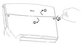
Step 1. Remove the front cover(s) from the base assembly.
