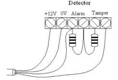
Wiring a single detector
