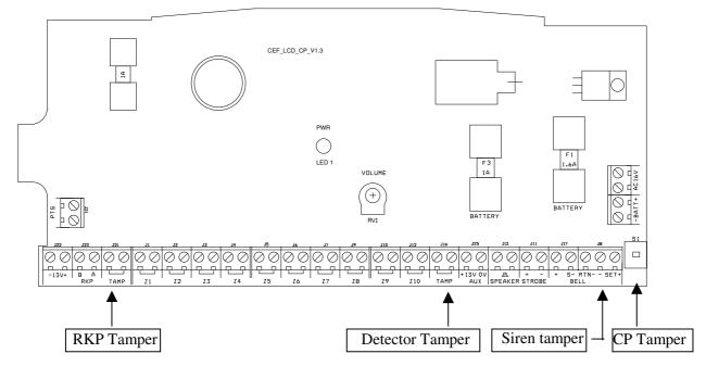
**CAUTION**: Always power-down the panel when wiring external circuits, to prevent damage to the panel electronics.
