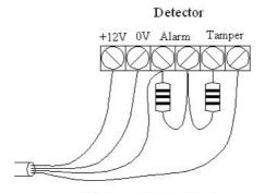
Wiring a single detector
