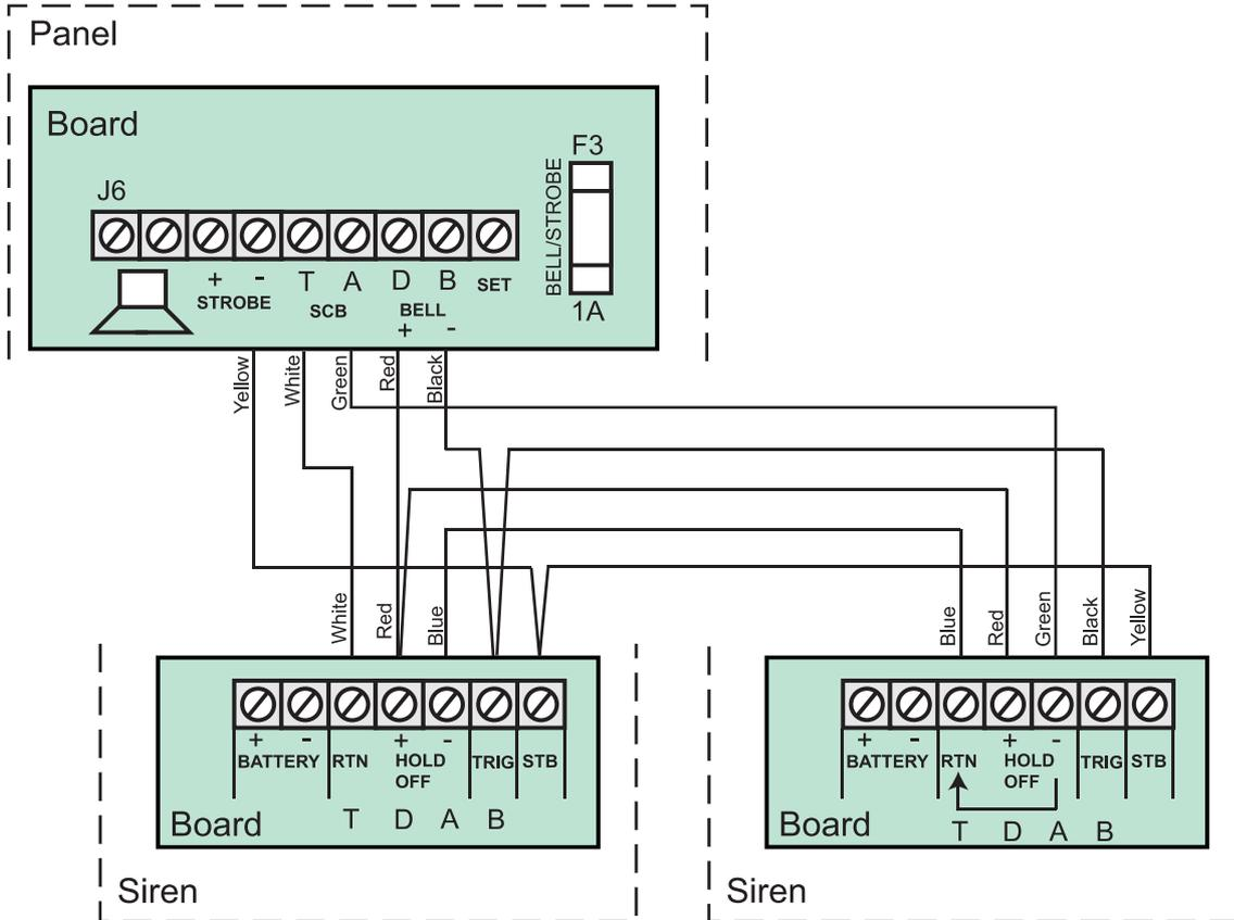
Figure 12. Twin External Siren Wiring
