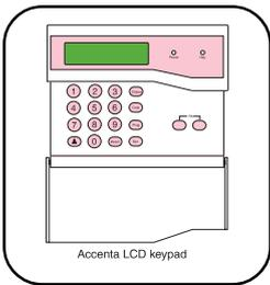
The **Remote Keypads (RKPs)** should be mounted in positions which allows ease of operation for the system users, typically within the entry/exit route close to the final door and the master bedroom.
