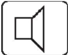
Additional internal **sound speakers** are recommended, these will provide high volume alarm tones and low volume entry/exit tones. Speakers should be positioned to provide good sound distribution throughout the building and so that the exit tone is audible outside the main entry / exit door. This will enable the system operator to check that the system is setting correctly.
