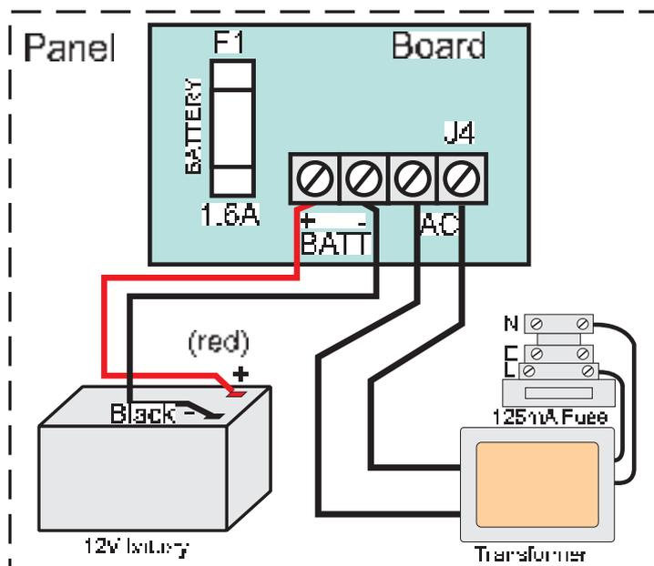
**Figure 15. Battery Connection**
