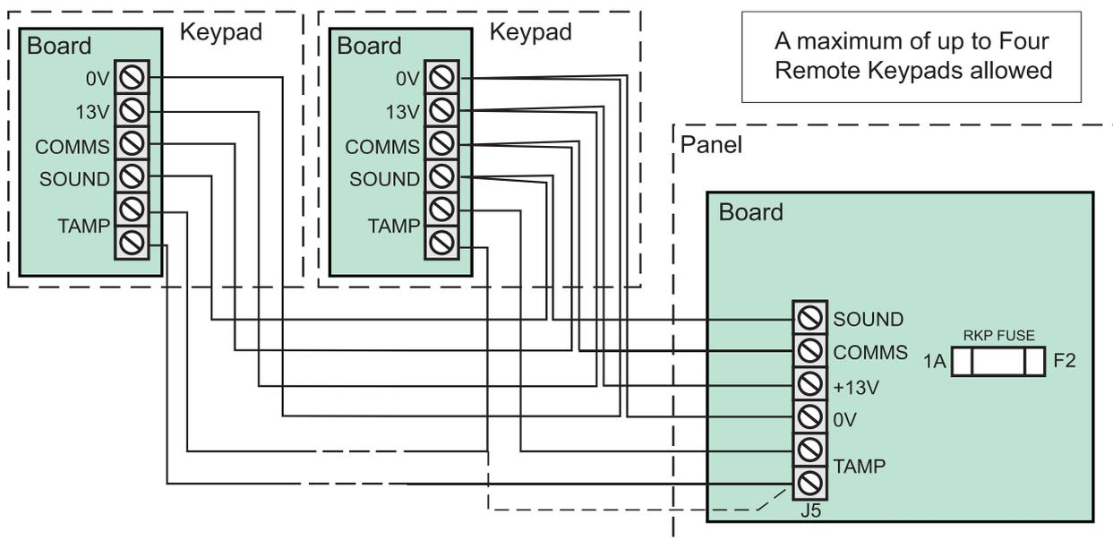
Figure 5. Connecting LED keypads to panel
