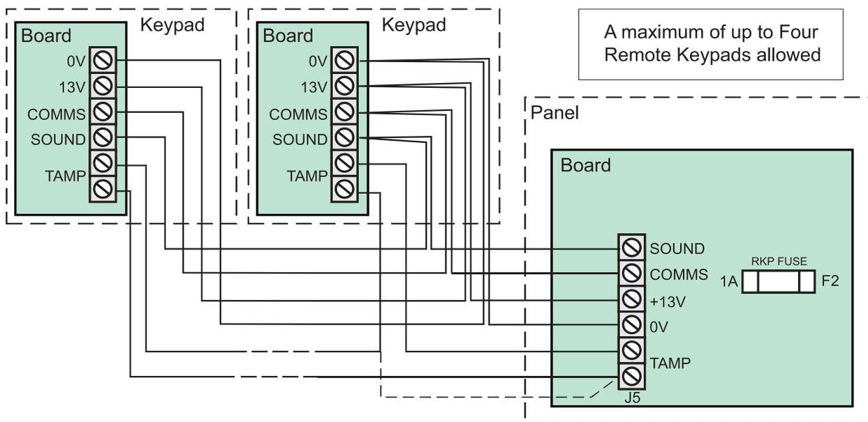
Figure 5. Connecting LED keypads to panel
