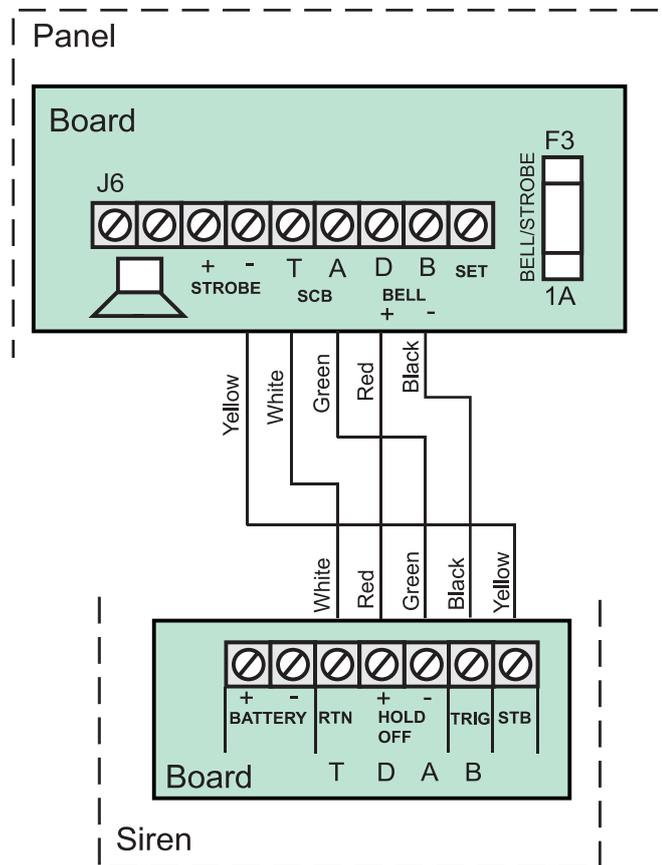
Figure 11. External Siren Wiring
