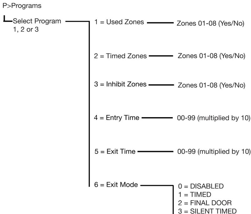
Figure 16. Programming structure
