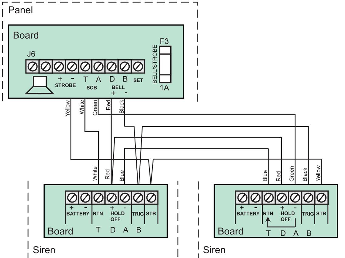
Figure 12. Twin External Siren Wiring
