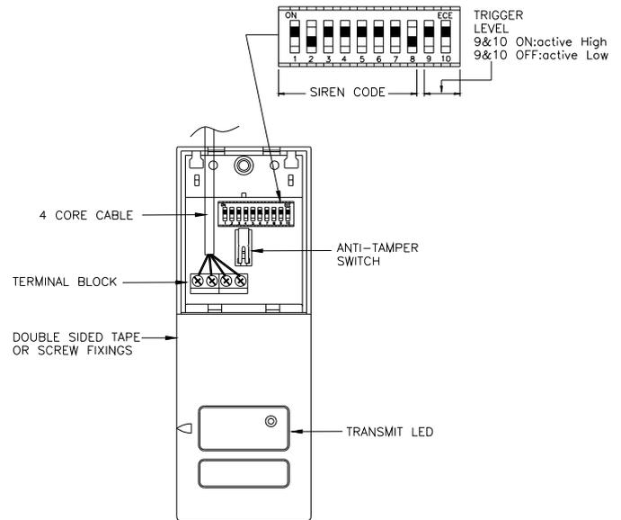
Undo the terminal cover screw and remove the terminal cover on the transmitter. REMOVE ALL POWER (MAINS AND BATTERY) FROM THE CONTROL PANEL. Lead the cable (option) to the control panel terminals and connect as follows:
