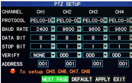
**CHANNEL:** selecting the channel to which the dome camera is connected (to select any of the latter 4 channels, click "Next Page")
