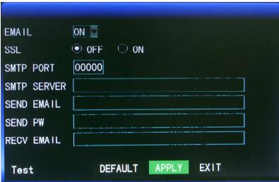
**SSL:** a secure link transmission protocol. "Off" is usually chosen.
