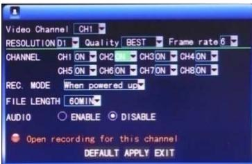
**Channel:** Select the corresponding video channel on or off (16ch DVR with 16 channels).
