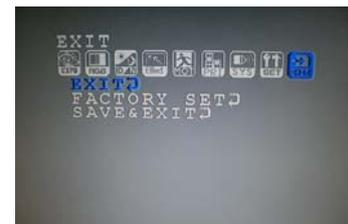
When all settings are complete, press "Up", "Down" to move the cursor to "Return", then press "OK", "Exit" dialog will turn up, select "Exit" (Exit menu, do not save the settings of parameters) or "factory original settings" (it means to recover factory settings) or "Save & Exit" (save the changes of parameters and then exit the menu) and then press "OK" to perform the corresponding return functions.
