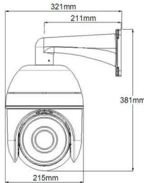
Pan 360° continuously, tilt 90° rotation, auto-flip, manual speed: 0.2°~200°/s.
