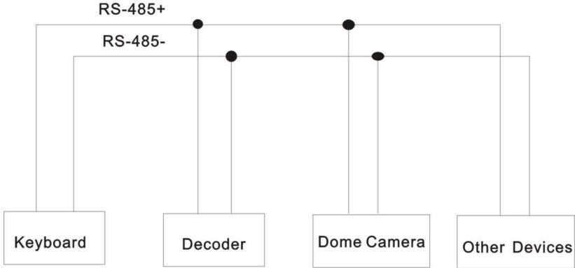
The control system of controlling multiple dome cameras is as below:
