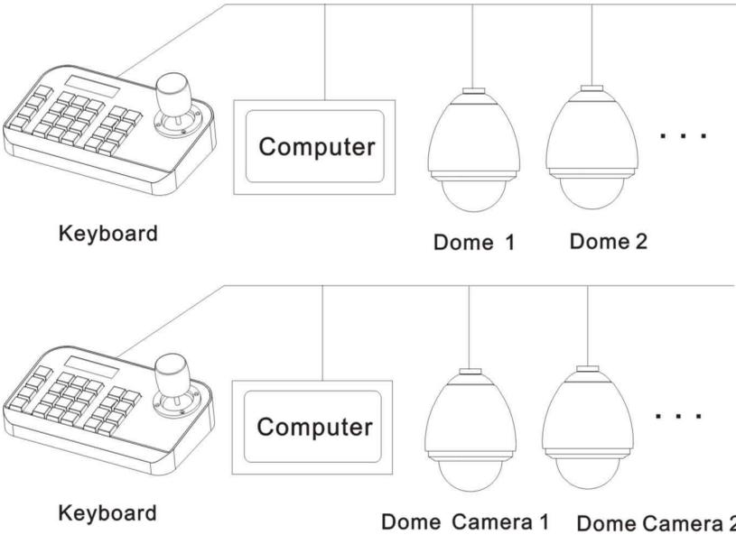
Notice: Before using the keyboard to control dome camera, please make sure the address, protocol, baud rate of the
