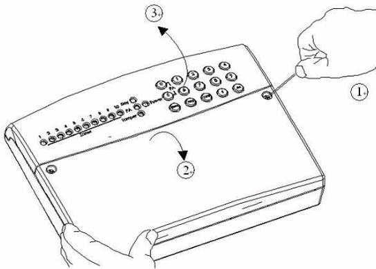
Step 1. Remove the front cover(s) from the base assembly.
