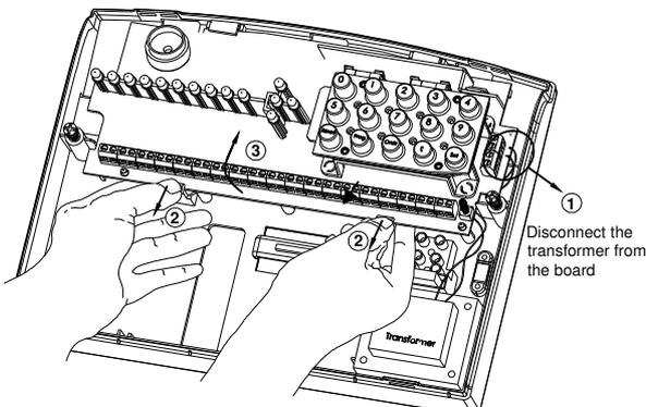
Disconnect the transformer wires from the board, these are marked AC. Carefully remove the board by gently pushing down the holding clips on the bottom edge of the board and with draw it from the base.
