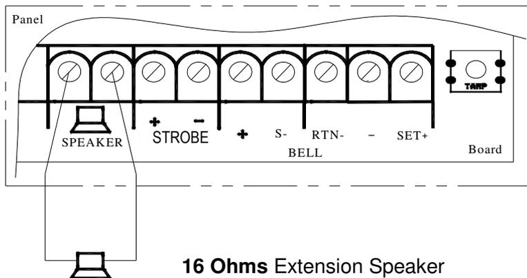
Only one 16 ohm extension speaker may be wired across the speaker terminals. Mounted in convenient position within the installation the extension speaker will reproduce all of the alarm tones generated by the control panel.
