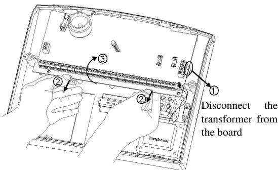
Disconnect the transformer wires from the board, these are marked AC. Carefully remove the board by gently pushing down the holding clips on the bottom edge of the board and with draw it from the base.
