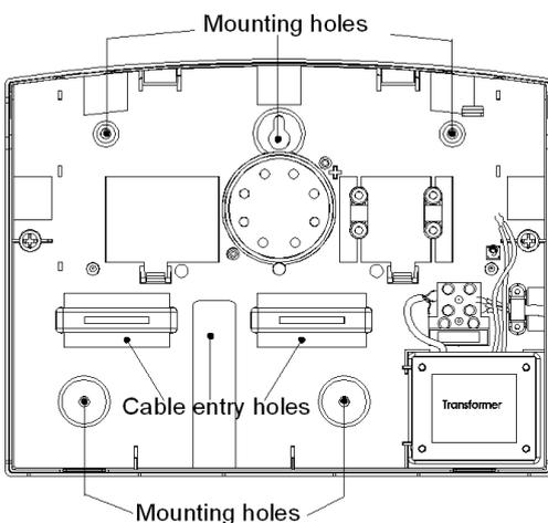
Step 2. Fit the panel to wall with suitable fixings. Ensure the wall surface is flat to prevent base distortion. There are cable entry holes provided in the rear of the base and around the outside edges through the thinned out plastic sections which may be cut away as required.
