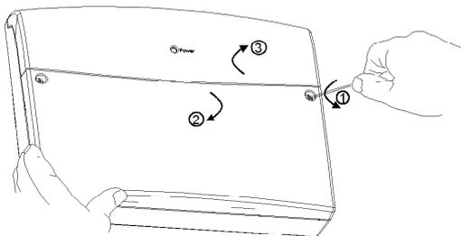
Step 1. Remove the front cover(s) from the base assembly.
