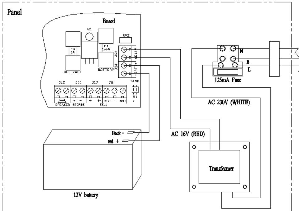
**CAUTION:** To avoid the risk of electrical shock you must always totally isolate the mains supply before opening the control panel cover(s).
