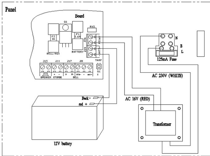
c. On connecting the battery the system will now go into alarm condition and Day led is will be lit.
