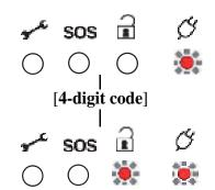
If any Zone, (Tamper) or sos (Attack) LED s come on then an alarm has occurred, and an intrusion may have taken place. Seek assistance before investigating further as intruders may still be on the premises. Then reset the system.
