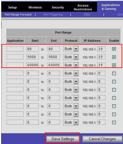
Put the DVR's IP and port (WEB port, media port, phone port) to fill in the corresponding location, the protocol is "Both", and the state is "Enable" or Reboot. Then click "Save Settings", add other ports in the same way. 6000 is mobile phone monitoring port, this port must be added in order to use the mobile phone surveillance function. As shown above, 9000,80 and 6000 port can all be modified in the DVR main menu.
