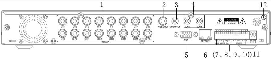
1. Video in 2. Video out (BNC port) 3. Audio out 4. Audio in 5. VGA output port
