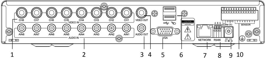
1. Video in 2. Audio in 3. Audio out 4. Video out 5. VGA output port 6. USB interface
