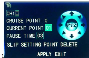
Operate the PTZ with mouse through the keypad on the interface. Set the cruise point in the cruise setup, as shown on the right picture above.
