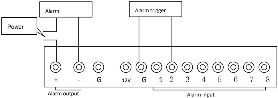
Note: The above picture is the type of normally on alarm, and normally off is the opposite way.
