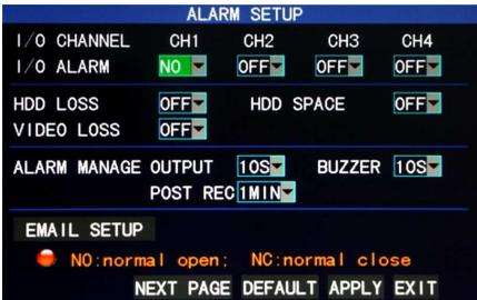
**ON:** indicating that external alarm circuit is open circuit without alarm but closed circuit with alarm.
