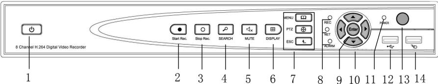
1.Power switch 2.Start recording 3.Stop recording 4.Video search 5.Mute 6.Display mode 7.Main menu; PTZ control; Exit/Return 8.LINK:Network connection indicator 9.Confirm 10.Direction 11.Power LED 12. 2.0 USB interface, which can be accessed to USB disk for backup or upgrading 13.Remote control infrared receiver 14.USB mouse interface
