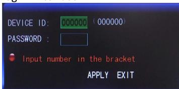
**Device ID:** It is just okay to enter device ID displayed on the right side in corresponding input box. The default ID will be guided when mouse operation is done. We recommend setting a password when remote controller is operating many types of equipment, to distinguish through targeted equipment code input, or the remote controller will disturb the adjacent mainframe.
