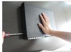
④ fix the screw of hard disk
