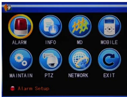
The advanced functions include the 7 options of alarm setup, system information, motion detection, mobile phone monitoring, system maintenance, PTZ Setup and Network Setup.
