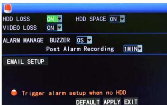
**HDD LOSS:** On: When the system cannot identify the harddisk, an alarm will be generated, and a red mark “H” will be displayed at the bottom left corner of Channel 1 in the lower part of the Video Preview screen.
