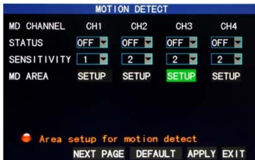
**MD Channel and STATUS:** Each channel has a corresponding switch. Press “Enter” to select motion detection “On” or “Off”.
