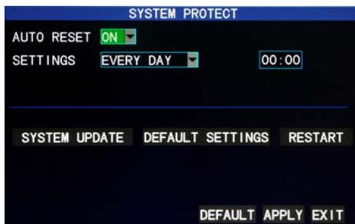
**AUTO RESET:** When this option is set to “On”, the user can set the restart frequency and time of this device himself/herself.
