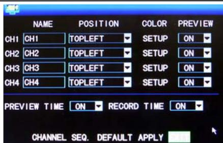
**Name:** Move the cursor to the input box of this option, and press “Enter” to enter the input screen of this option. Numerical, English and Chinese pinyin input methods are supported;
