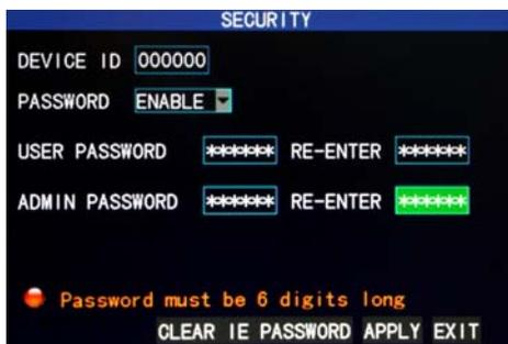
**DEVICE ID:** Enter digits directly to set up the DVR number;
