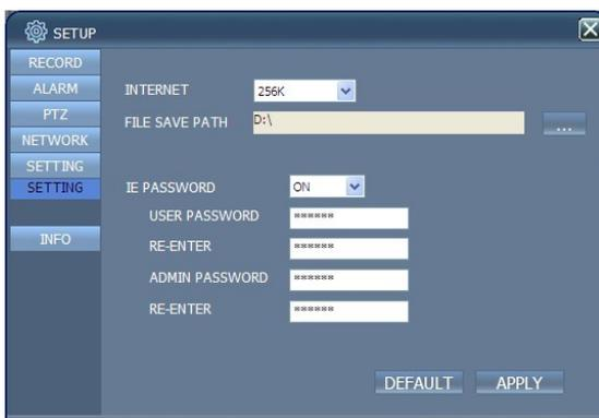
**INTERNET:** setting the code stream; the higher the code stream is, the clearer the remote image will be, but the network bandwidth must be high, otherwise the image may have a delay.
