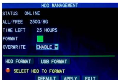
**STATUS:** After the hard disk is connected, the system will detect if the hard disk is correct automatically. If the hard disk needs formatting, "Unformatted" will be displayed in the hard disk state, when you can click "HDD Format" to format the hard disk. If the system detects any available hard disk, the hard disk state will be "ONLINE";
