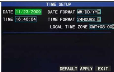
The system time, date format, time format, time zone and summer time can be set up in this screen.
