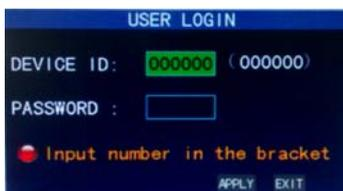
**Equipment code:** it is just ok to enter equipment code “000000” displayed on right side in corresponding input box. The defaulted code will be guided to the number box when mouse operation; we recommend to set mainframe password when remote controller is operating many equipments, to divide through targeted equipment code input, or the remote controller will disturb the adjacent mainframe.
