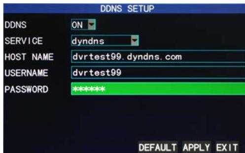
**DDNS (domain name resolution):** with the two options of "ON" and "OFF"; when a domain name resolution server is available, please select DDNS "ON";
