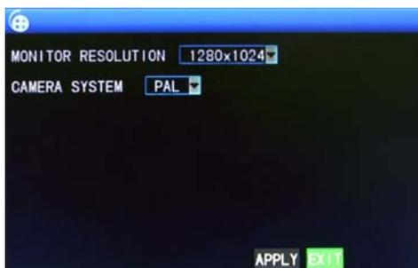
**MONITOR RESOLUTION:** Left-click or press “Enter” to set the VGA output resolution, with the 3 options of 1280\*1024, 1024\*768 and 800\*600;
