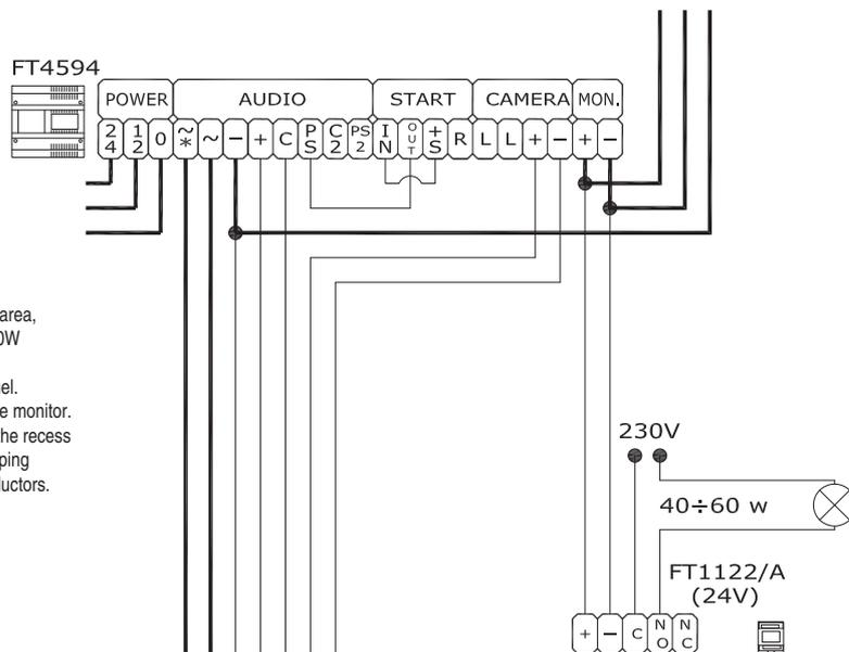
If the external unit is placed in a totally dark area, we recommend installing an additional 40-60W lamp mains voltage controlled by a relay FT1122/A, at 30 cm above the entrance panel. The lamp will light up at the same time as the monitor. Conductors for the lamp must not be run in the recess box of the entrance panel nor through the piping containing the video door entry system conductors.
