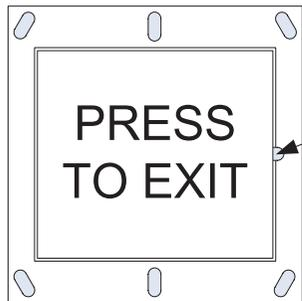
TO ACCESS 1 GANG MOUNTING HOLE USE SMALL DRIVER TO REMOVE THE BUTTON
