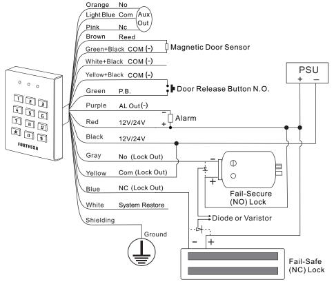
A DC power supply is required for Fail-Safe locks
