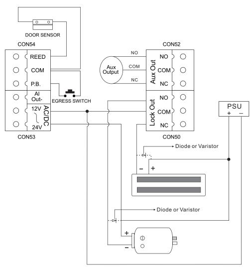
A DC power supply is required for Fail-Safe locks
